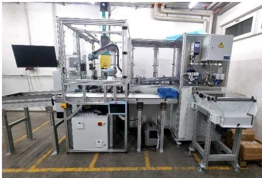
Image 2: Al-pro developed a system to compress ball sleeves automatically. The forming is performed by a stable servo press from TOX PRESSOTECHNIK, which is initially configured once, or in case of a part replacement via the TOX-HMI. The Al-pro automation then issues the start and stop signal.
