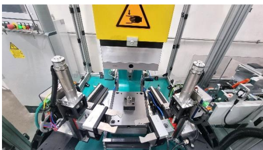
Image 3: Two linear-guided grippers alternately insert a component into the tool of the TOX-Servopress and remove it after pressing.
