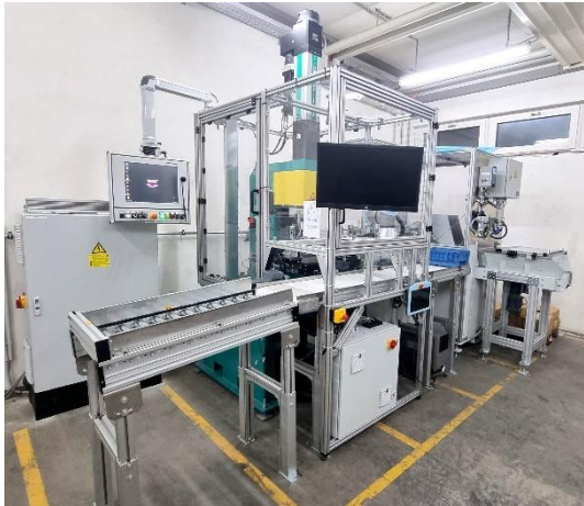
Image 1: Al-pro selects a C-frame press from TOX PRESSOTECHNIK GmbH & Co. KG for the automated compression of ball sleeves and complements it with the required handling and sorting units.
