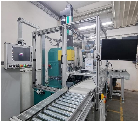
Image 6: The TOX-ElectricDrive drive is installed in a solid and torsion-resistant steel structure, which meets the force application with sufficient stability during the pressing process.
